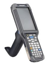
Built on the Honeywell Mobility Edge platform, the ultra-rugged CK65 mobile computer combines touchscreen and keypad data input, real-time connectivity, and advanced data capture for industry-leading investment protection.
